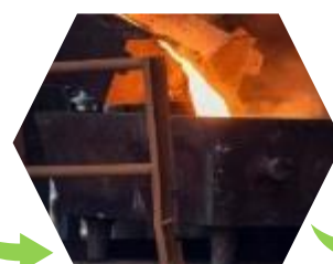
Waste melting at furnace exit 1.500°C
